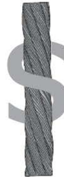
Left hand lang's lay (LHLL/LHL/sS)
