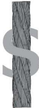
Left hand regular lay (LHRL/LHO/zS)
